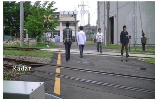
Fig.12 Detection of multiple human experiment in crossing.
