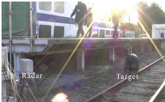
Fig.10 Experiment to detect the fall from the platform.
