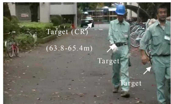
Fig.8 Detection of CR and multiple human experiment.
