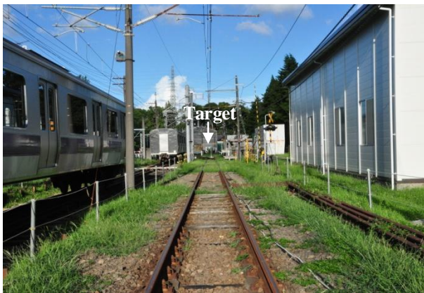
Fig.15 View from the train equipped with the radar at about 30km/h (about 80m from the target)
