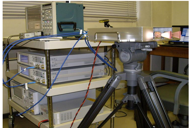
Fig.9 Outline view of 24GHz radar
