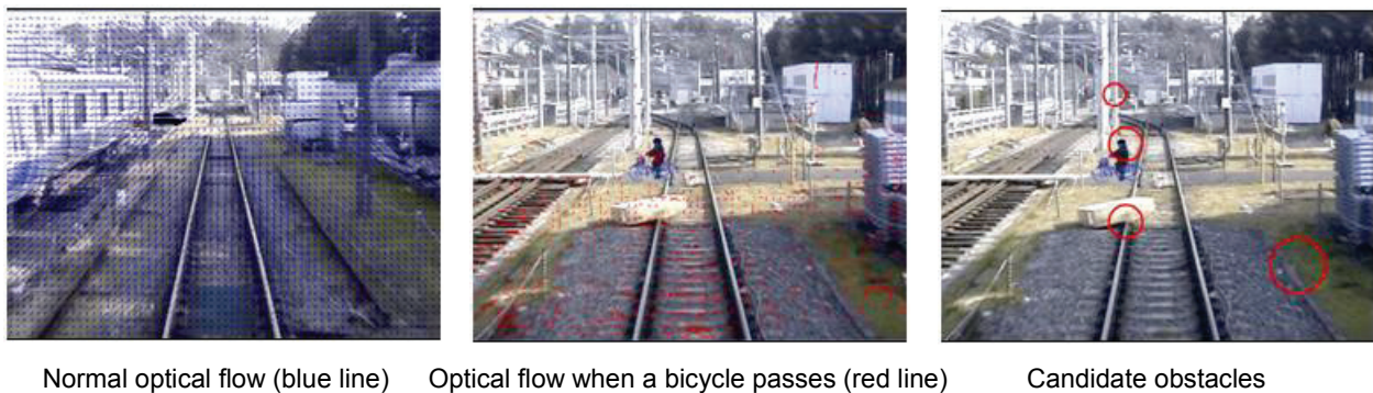
Figure 12. Results of obstacle detection using optical flows
